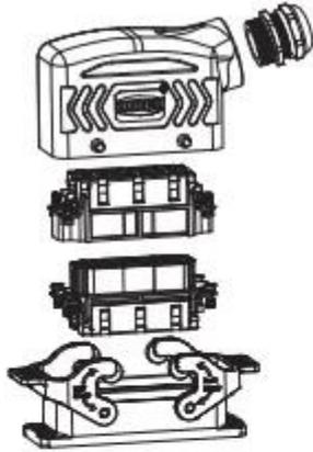
● 开孔安装/Bulkhead mounting
