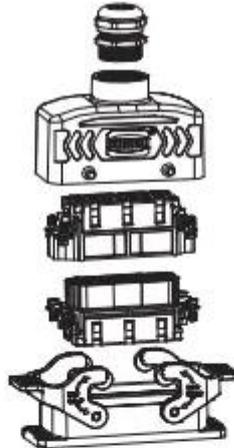
● 开孔安装/Bulkhead mounting
